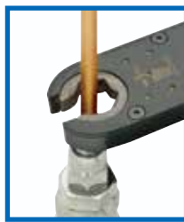
Push lever in the middle position, confirm socket in open position.
